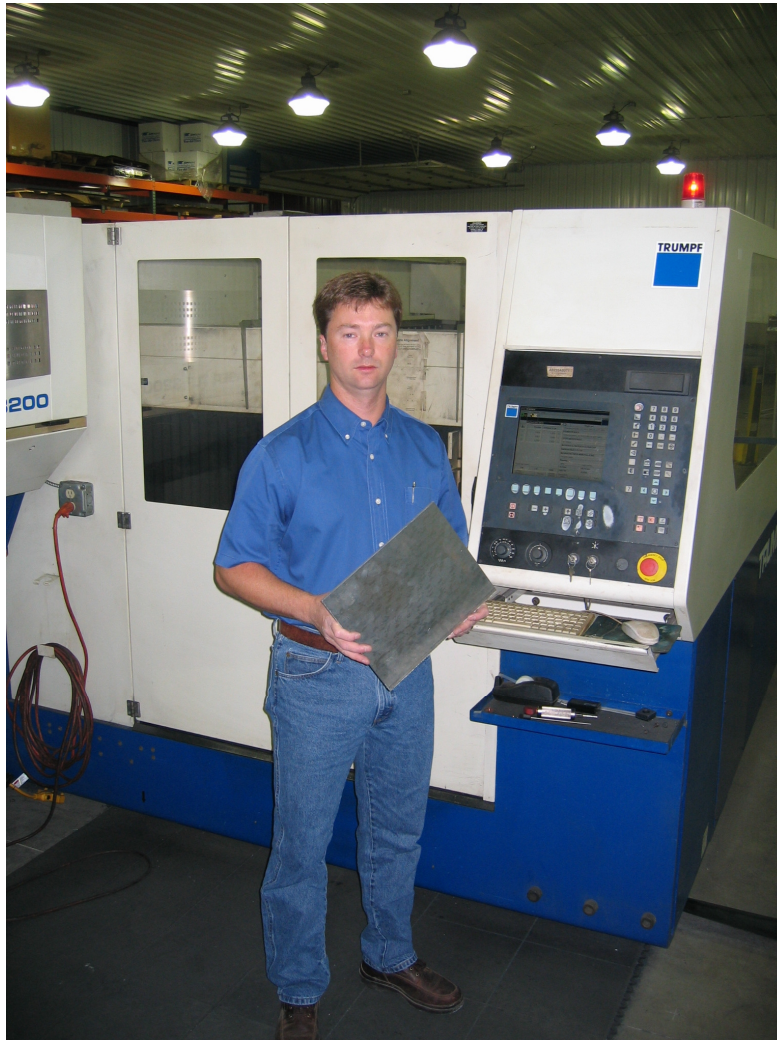
Figure 1: Jason Greeson, Fab 2 Order, with a piece of .357" thick 5052 Aluminum cut at 16" per minute. This represents a 78 percent increase over stock parameters for a 3200W Trumpf.
